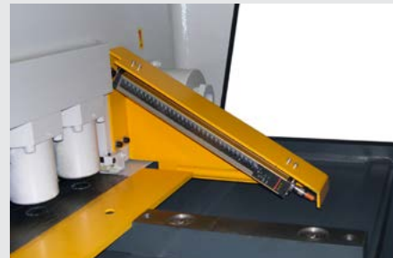
SAFETY LIGHT CURTAIN GUARDS in front of the hold-downs. BALL TRANSFERS mounted in the iron table blocks, for easy feed-in of the sheets. blocks, for easy feed-in of the sheets.
